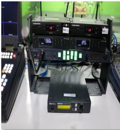
DATA VIDEO AUDI DELAY UNIT MODEL NO: AD-100M & DATA VIDEO FEEDBACK SYSTEM
